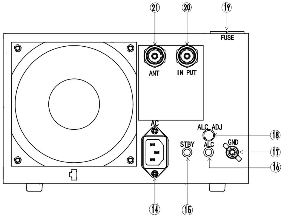
**AC POWER** : AC Mains Socket. Socket for the AC power cord. (Socket is EMI filtered.)
