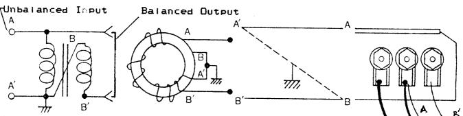
Wind 2 wires in parallel over the core. The core used is a T-200-2 type toroidial core by AMIDON. 1mm diameter magnet wire (or enameled wire) is wound 15 times (about 3m long x 2wired) in bifilar fashion over the core. The core is rated up to 1kw input. Maximum power input is figured by the following calculation. —— Balun coil diameter  $(T-200) \times 5 = 1$ kw. Putting insulating tape or glass tape produces an even better result. This balun is not provided.
